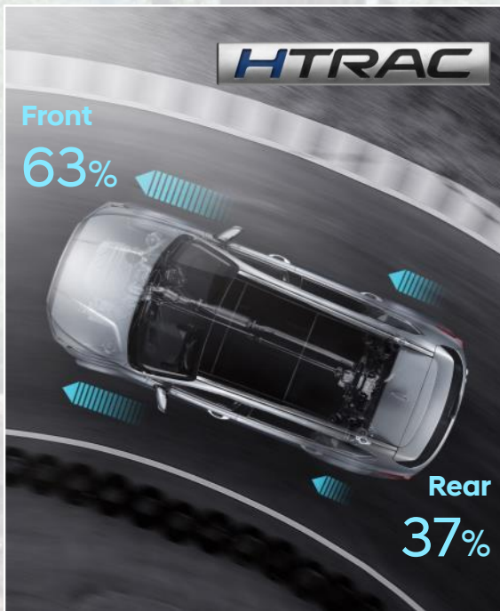
HTRAC driving force distribution by drive mode
