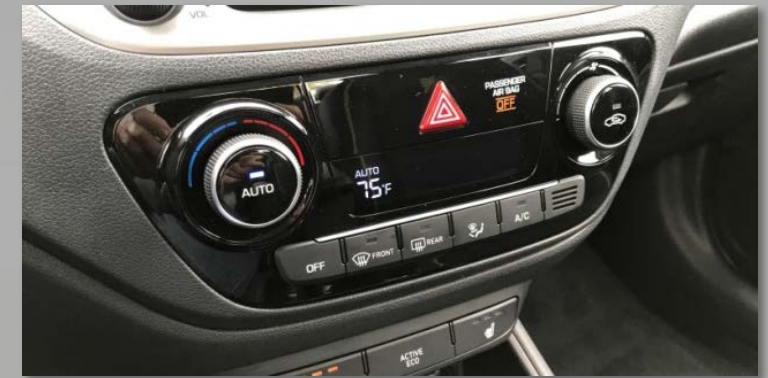
Automatic Temperature Control
